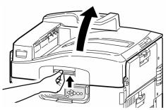
3. Pull the fuser lock lever as shown to unlock the fuser.
